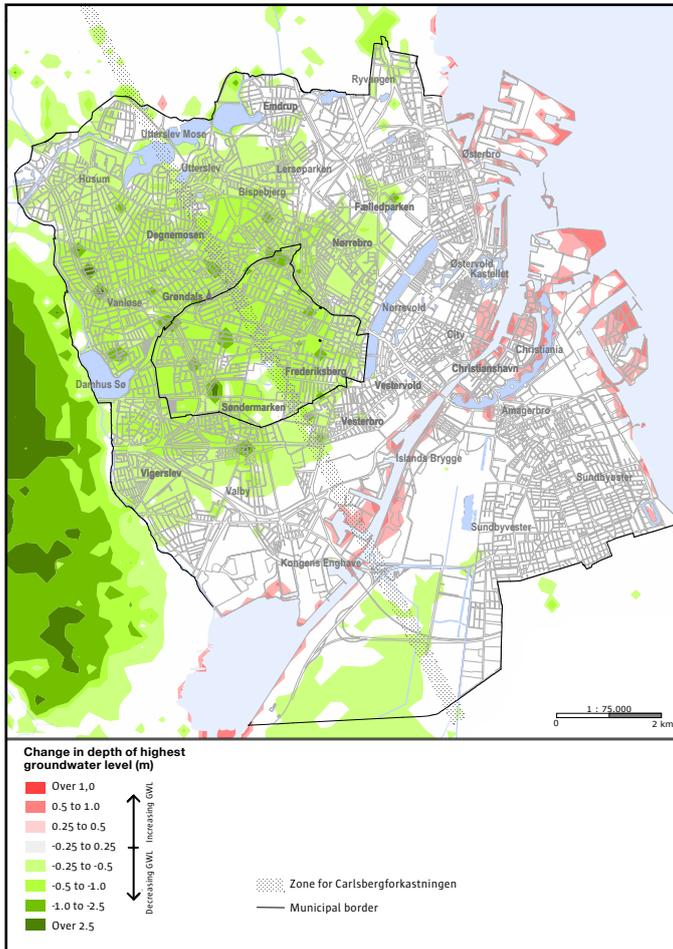
Figure 2: Change in depth of highest groundwater level—2110.
